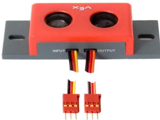
Figure 9 Ultrasonic range finder (VEX, 2016)
